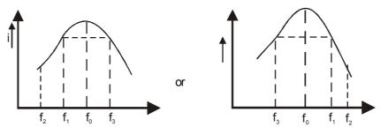
$\begin{array}{l} f_{_{0}} \text{ is resonant frequency} \Rightarrow \text{ means same as circuit being resistive.} \\ \text{The circuit is capacitative when } f < f_{_{0}} \text{ and inductive when } f > f_{_{0}} \\ \text{Power at } f_{_{1}} \text{ and } f_{_{3}} \text{ same} \Rightarrow \text{ i same} \Rightarrow z \text{ same} \end{array}$
